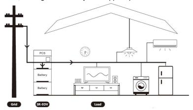
When the mains is disconnected or stops working, the battery supplies power to the load through the power module.
