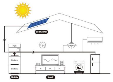
At night, the battery supplies power to the loads through the power module.
