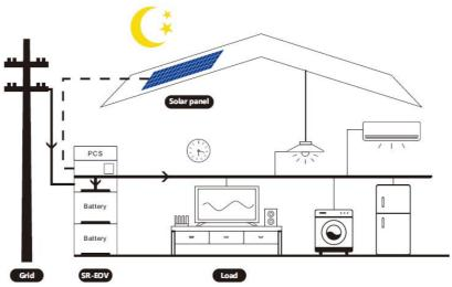
If the mains is disconnected, the battery supplies power to the loads.
