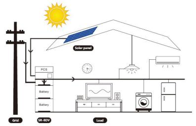
At night, the mains supplies power to the loads, and continues to charge the battery, if the battery is not fully charged.
